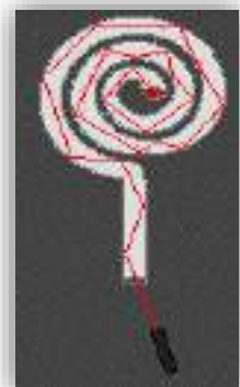
Critical Angle ( \theta_c ) is the largest angle of incidence for which refraction can occur
